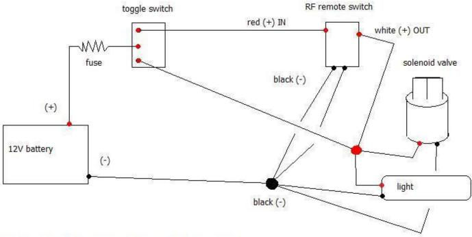
Note: Toggle switch is in small electric box near base of auger.
